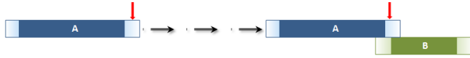
Figure 16: Temporal entity A ends before or with the start of temporal entity B. Here A is longer than B
