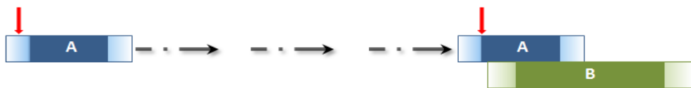
Figure 15: Temporal entity A starts before the start of temporal entity B. Here A is shorter than B
