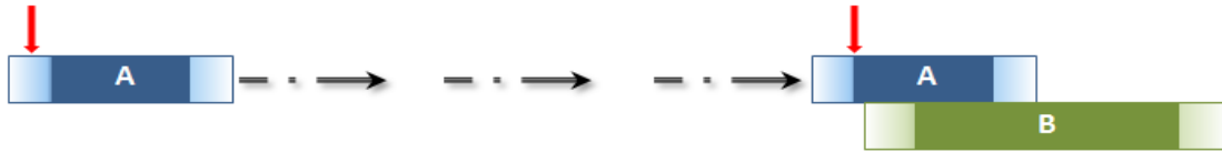
Figure 8: Temporal entity A starts before the start of temporal entity B. Here A is shorter than B
