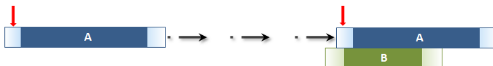
Figure 21: Temporal entity A starts before or with the start of temporal entity B. Here A is longer than B
