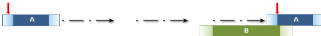
Figure 20: Temporal entity A starts before the end of temporal entity B. Here A is shorter than B
