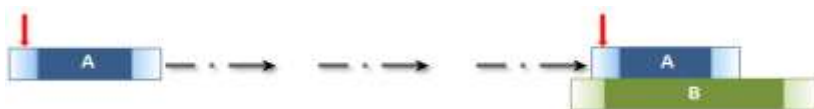
Figure 6: Temporal entity A starts before or with the start of temporal entity B. Here A is shorter than B
